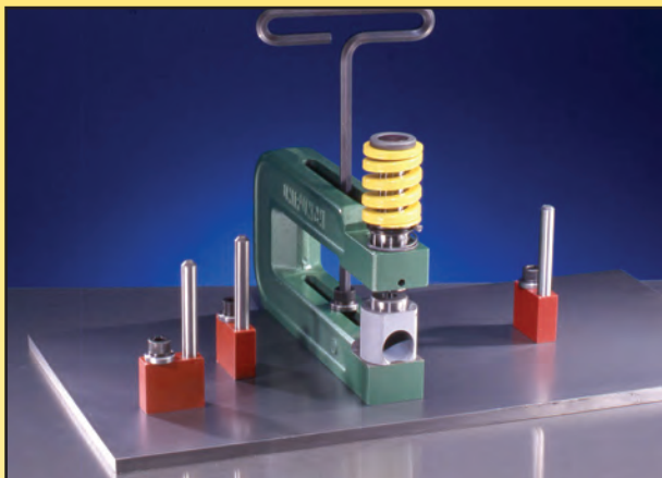
Typical 3-pin gauging Template Mounting
