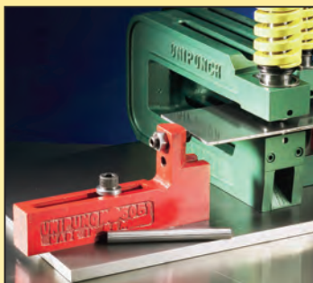
Typical 3-pin gauging Template Mounting
